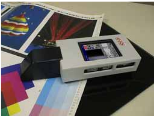
Fig. 6 DIAS – Distinctness of Image Analysis System
