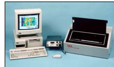
Fig. 4 DRA-2000L Dielectric Relaxation Analysis System
